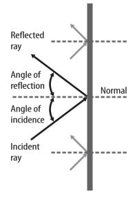
side of the normal. This angle is the angle of reflection. According to the **law of reflection**, when a wave is reflected from a surface, the angle of reflection is equal to the angle of incidence.
